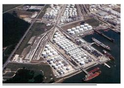
242 tanks for oil and petrochemicals with capacity of 1,115,100 m<sup>3</sup> (1 003 590 tonnes)
